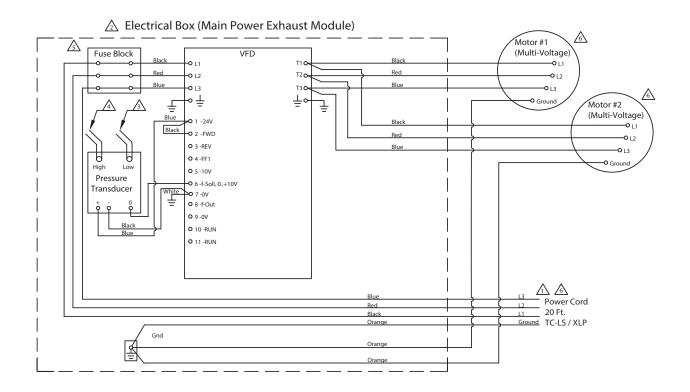
Power Supply. Provide disconnect means and circuit protection as required. See power exhaust name plate for electrical ratings. If local codes allow connecting to the HVAC unit power, make sure the disconnect and incoming wiring are sized to handle the load of both the HVAC unit and the power exhaust.
