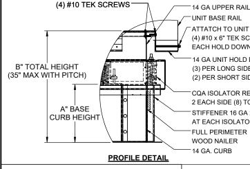
UNIT BASE RAIL ATTATCH TO UNIT WITH (4) #10 x 6" TEK SCREWS EACH HOLD DOWN 14 GA UNIT HOLD DOWN (3) PER LONG SIDE (2) PER SHORT SIDE CQA ISOLATOR RESTRAINTS 2 EACH SIDE (8) TOTAL STIFFENER 16 GA x 7" x 1 1/2" AT EACH ISOLATOR FULL PERIMETER WOOD NAILER 14 GA, CURB
