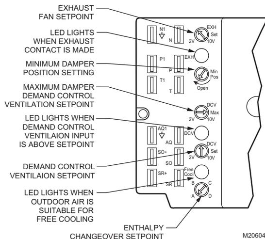
Fig. 6. Potentiometer and LED locations (W7212 shown).
