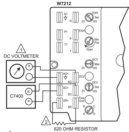
1 INSERT DC VOLTMETER BETWEEN AQ AND AQ1 FOR CHECKOUT AND TROUBLESHOOTING.
