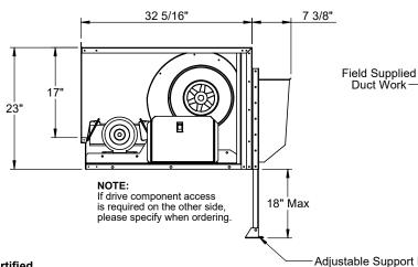
Drive Acces NOTE: Based on field supporting Adjustable Support Legs included of duct, P.E. may require additional field support.
