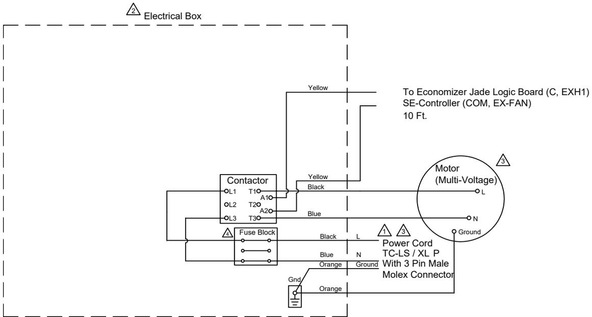
1 Power Supply. Provide disconnect means and circuit protection as required. See power exhaust name plate for electrical ratings. If local codes allow connecting to the HVAC unit power, make sure the disconnect and incoming wiring are sized to handle the load of both the HVAC unit and the power exhaust.
