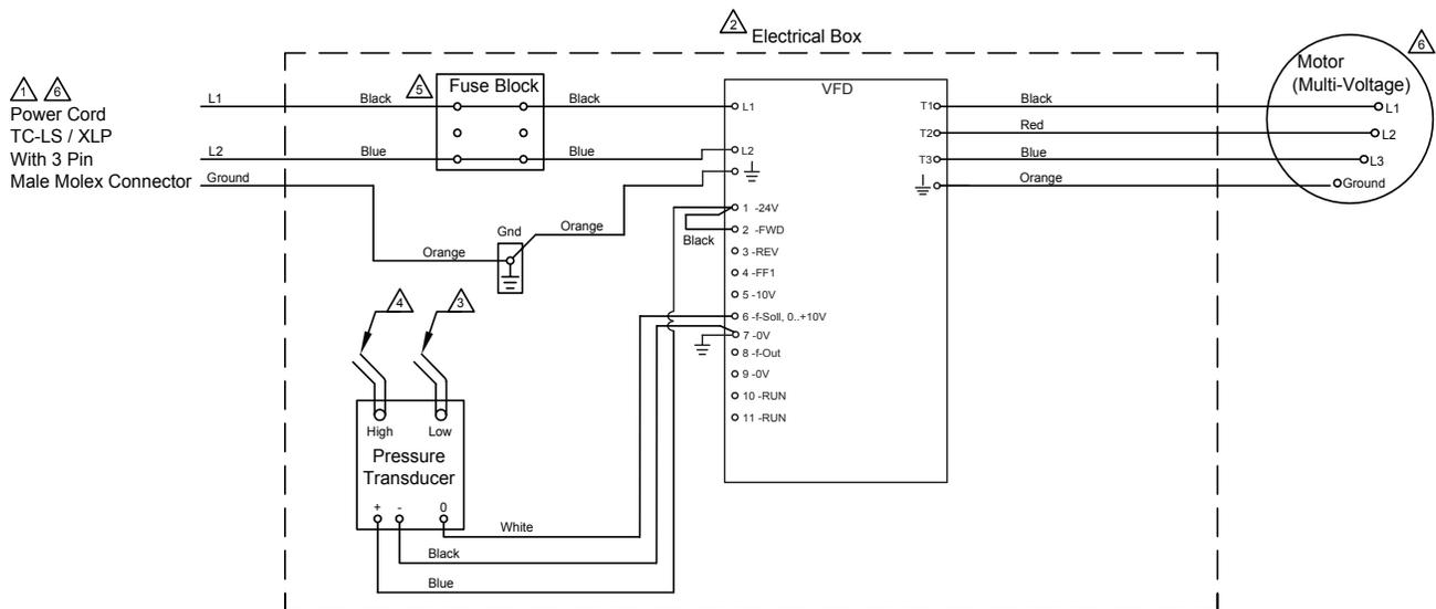
**⚠** Power Supply. Provide disconnect means and circuit protection as required. See power exhaust name plate for electrical ratings. If local codes allow connecting to the HVAC unit power, make sure the disconnect and incoming wiring are sized to handle the load of both the HVAC unit and the power exhaust.
