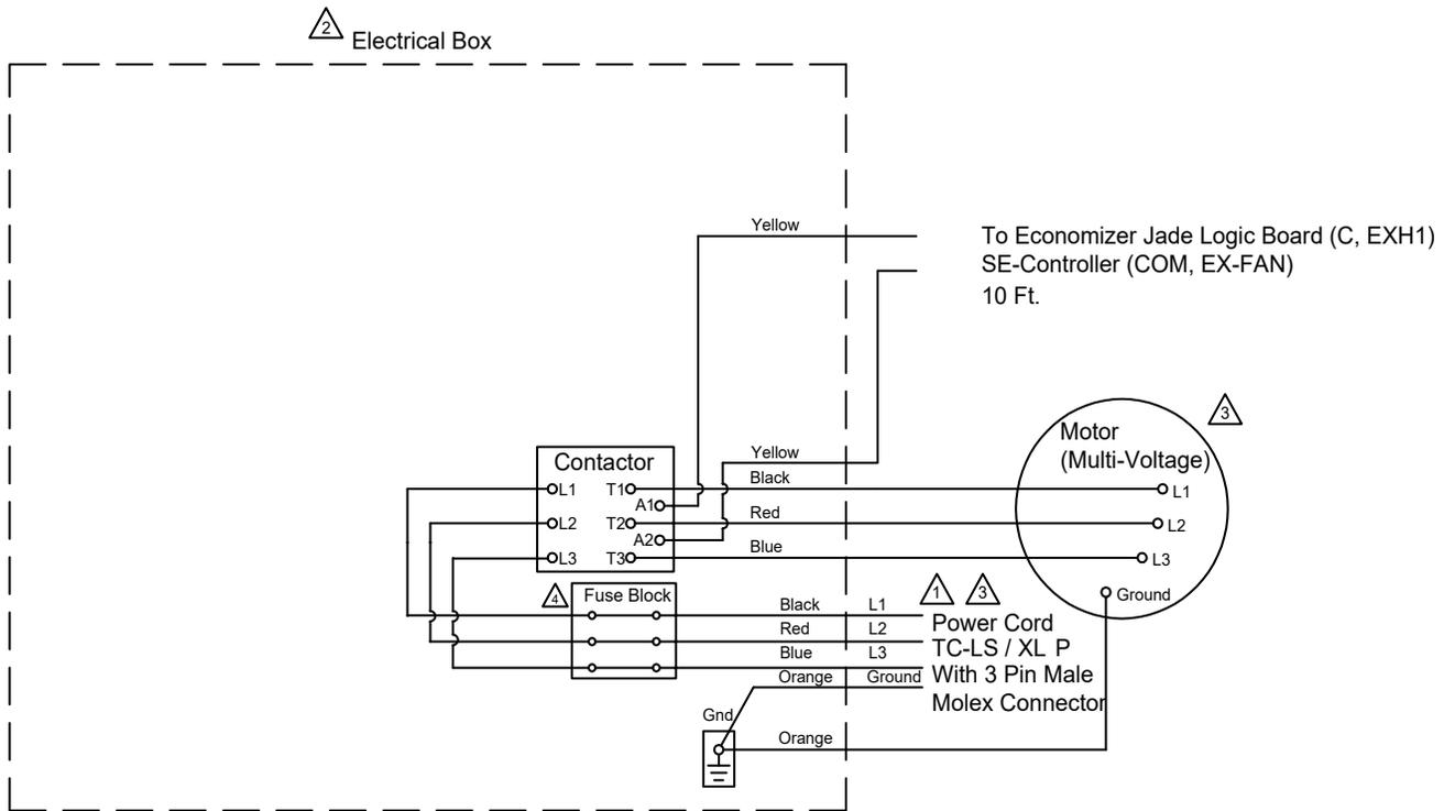
⚠️ Power Supply. Provide disconnect means and circuit protection as required. See power exhaust name plate for electrical ratings. If local codes allow connecting to the HVAC unit power, make sure the disconnect and incoming wiring are sized to handle the load of both the HVAC unit and the power exhaust.
