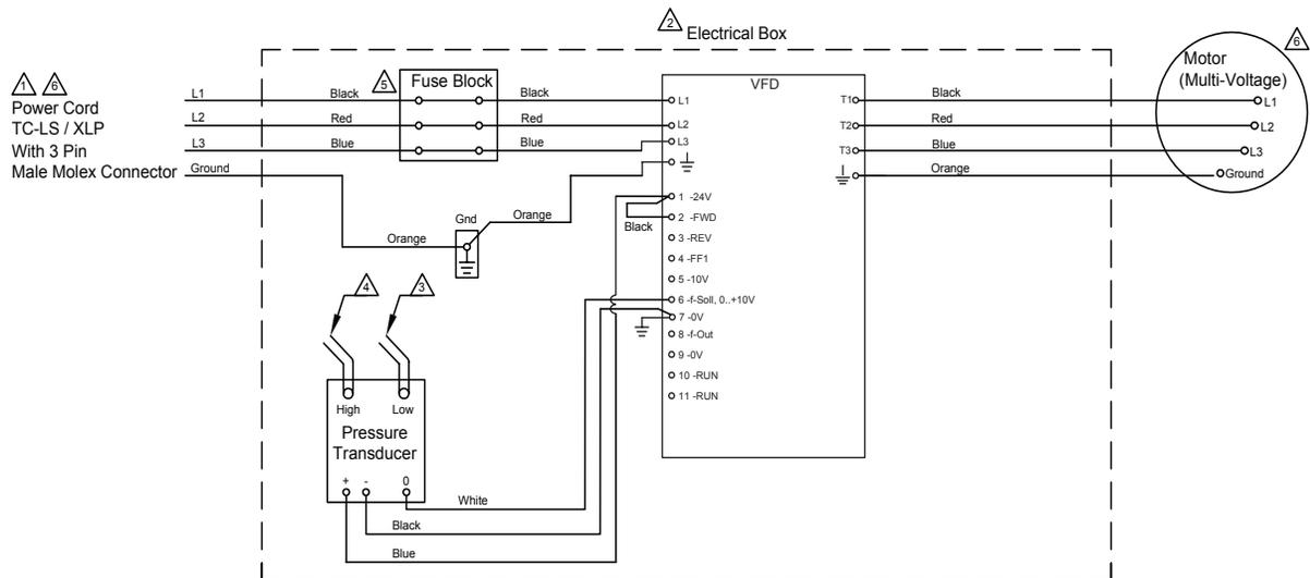
**⚠** Power Supply. Provide disconnect means and circuit protection as required. See power exhaust name plate for electrical ratings. If local codes allow connecting to the HVAC unit power, make sure the disconnect and incoming wiring are sized to handle the load of both the HVAC unit and the power exhaust.
