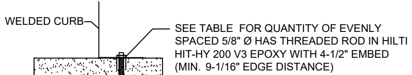
NO. OF ANCHORAGE BOLTS REQUIRED
